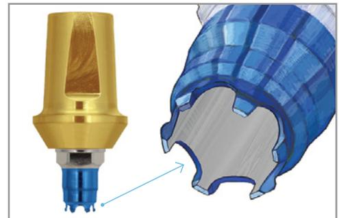
The 6/12 hex inside the internal connection incorporates both a 6-point single and a 12-point double hex. The 6-point single hex is designed for two functions: engaging the driver tip for mountless delivery during implant placement and providing anti-rotation for all straight abutments.
