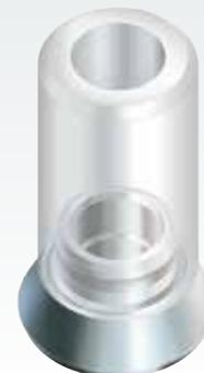
The gold base is fabricated from a non-oxidizing alloy that promotes chemical adhesion of the cast alloy, but does not permit the adhesion of porcelain. Therefore, a porcelain bonding alloy must be added to all areas of the gold base where porcelain veneering is desired.
