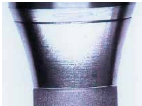
Transition between machined collar and textured surface of Tapered SwissPlus Implant.
